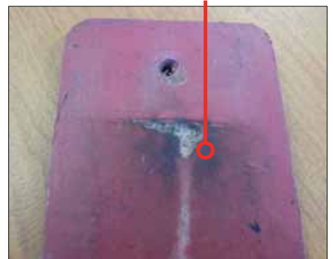
Erosion – Test sample passed the TERT test.
