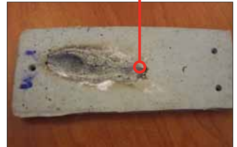
Tracking – Test sample failed during the TERT test.
