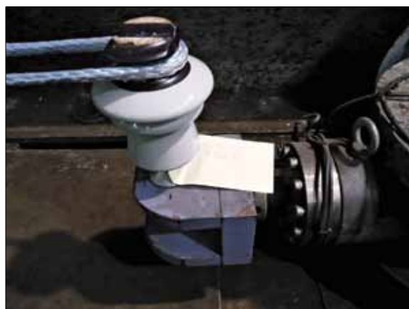
Testing cantilever strength of insulator pin.
