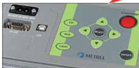
Intuitive keypad and connectivity to PC through RS 232 and USB
