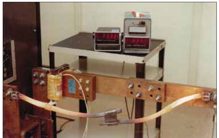
AMPACT Connector unique spring ability, reduces resistance and remains cooler.
