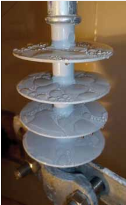
Polymer strain insulator during accelerated weathering
