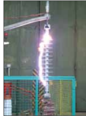
Polymer strain under the steep-front impulse voltage test
