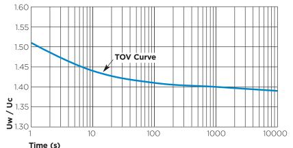
Temperature of samples (pre-heated): 60° C according to IEC 60099-4, Ed 2.0 2004. TOV Curve applies to an arrester which has a pre-stress applied prior to TOV verification. This prestress is equivalent to one high current impulse of 65 kA, 4/10 µs as per the switching surge operating duty test.
