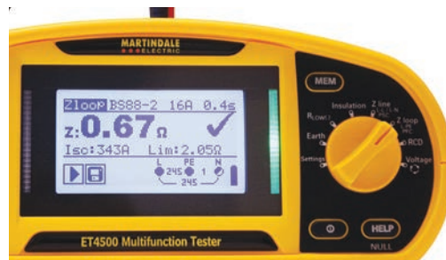
Pass/fail testing to the latest loop impedance limits.
