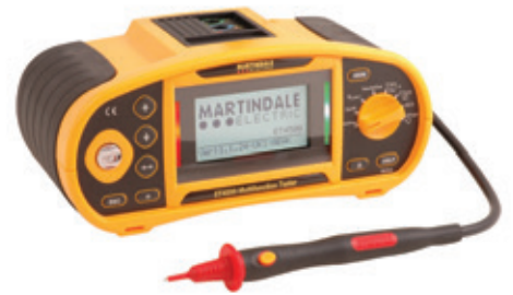
ET4500 PRO Downloading multifunction 17th Edition installation tester with memory, download and upload capability and 3 wire earth tester built-in Page 5
