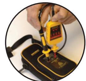
Re-prove the voltage indicator using a proving unit.
