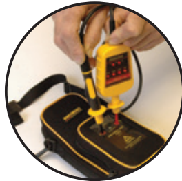
Prove your voltage indicator using a proving unit.
