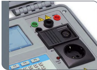
Connector panel - test ports for fixed installed appliances.
