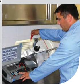
The multifunctional portable test instrument SigmaGT is intended to perform all measurements for testing the electrical safety of portable electrical equipment. The operation of the unit is clear and simple, the operator does not need any special training to operate the instrument. The instrument has a powerful test data management system where auto tests and single tests can be stored in approximately 6000 memory locations.
